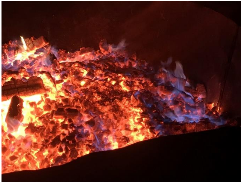
(Left), Some larger chunks on the top not burned emitting yellow flame, (Right) blue flame means it's cooked into biochar
