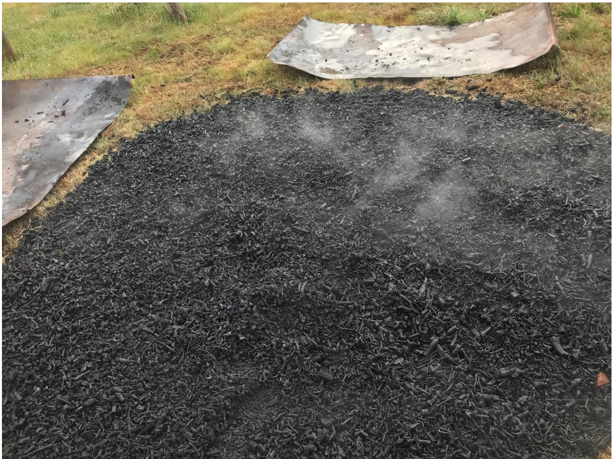
Fully quenched pile that is steaming, steam can also be a sign of a hot spot and should be investigated.
